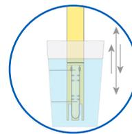
**Why** – Air can become trapped inside the probes or stay on the surface of the probes when they are submerged. This can cause erratic or erroneous readings.
